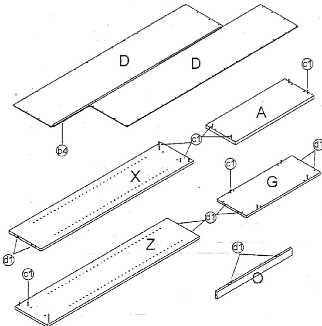
1. Insert cam bolts (c1) and dowel pins (d1) into panel A, G, X and Z as illustrated above.
