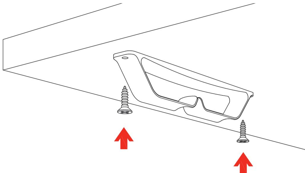
Screw fix to the underside of the desktop.
